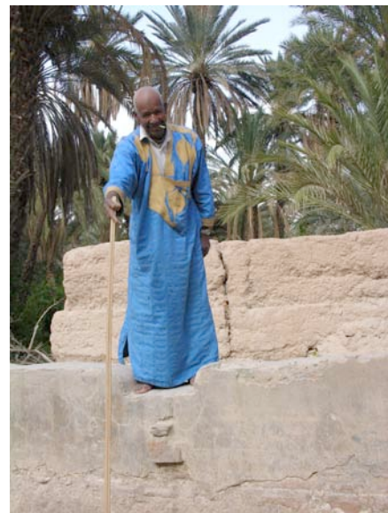
Measuring water level in the basin for equal distribution.
